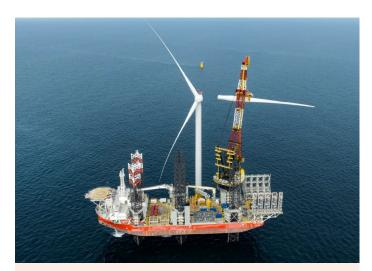
Cadeler's offshore wind turbine installation vessel
